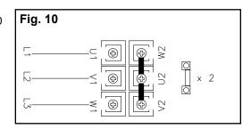
If the application requires 3x208-240VAC operation, the jumper positions must be changed according to Fig. 11.
